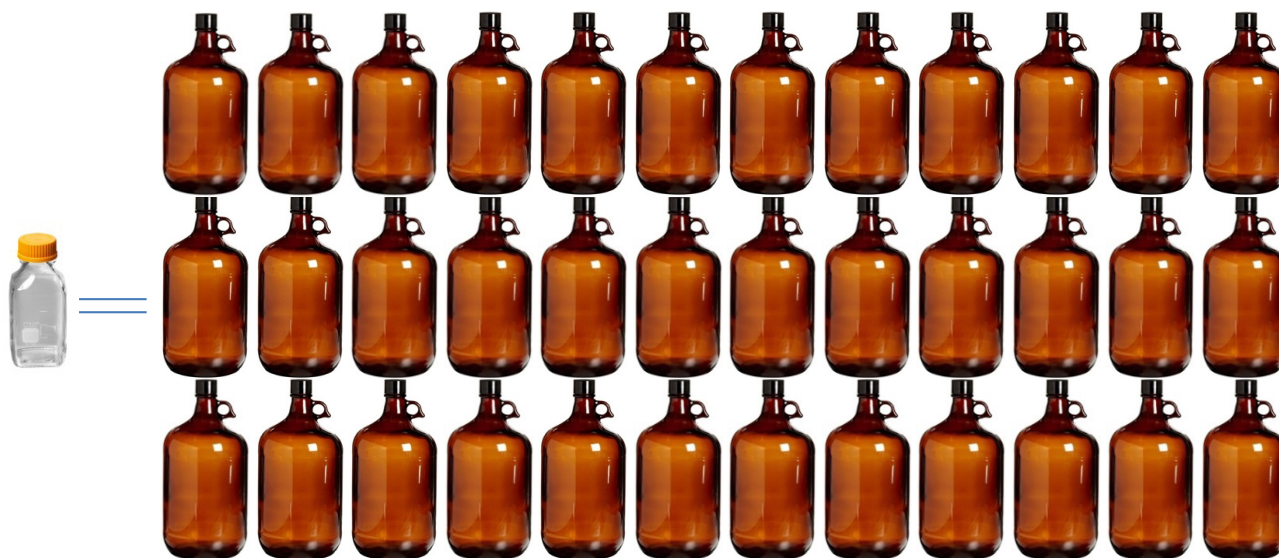
Figure 9. Comparison of relative solvent consumption of ionKey running at 7 \mu\text{L}/\text{min} flow rate vs. analytical scale chromatography running at 1 \text{ mL}/\text{min} flow rate is displayed. The figure shows that consuming 1 L solvent on the ionKey/MS System running continuously at 7 \mu\text{L}/\text{min} for 99 days or 35,700 injections at 4 min run time, is equivalent to thirty six 1-gallon bottles using an analytical scale system.
