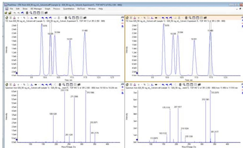
Figure 3. Recorded product ion spectra of prostaglandin D<sub>2</sub> (PD<sub>2</sub>) and dihydroketo PD<sub>2</sub> shown in PeakView<sup>®</sup> Software. The three most intense fragment ions were chosen for the quantitation method.
