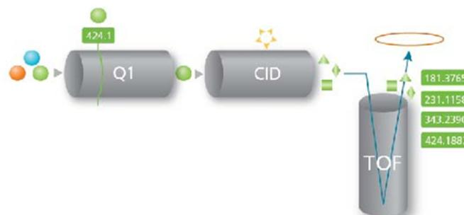
Figure 1. Schematic overview of MRM<sup>HR</sup> acquisition technique on a TripleTOF<sup>®</sup> System compared to standard triple quadrupole mass spectrometer.
