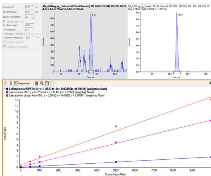
**Figure 5. Processing of calibration data for isoprostane species.** MultiQuant™ Software was used to measure peak areas corresponding to MRM<sup>HR</sup> signals (top). Calibrations curves are shown for standards for isoprostane species, 5-iso-prostaglandin F<sub>2α</sub>, prostaglandin D<sub>2</sub>, and dihydroketo prostaglandin D<sub>2</sub> (bottom).
