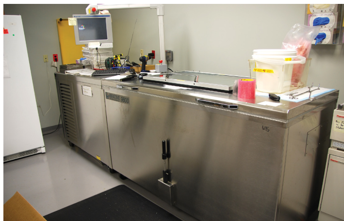
Figure 3. A typical cryomacrotome, used for sectioning animals in QWBA.
